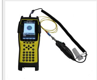
Figure 3: ARGUS 260 fiber multitester/multimeter for GPON-TE and PON installation tests, here with video microsope for optical inspection of glass fibers.
