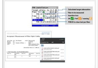
Figure 2: Example of a measuring wizard in an instrument (top) and an acceptance measurement log in PDF format on a PC (left) and a smart phone (bottom right).
